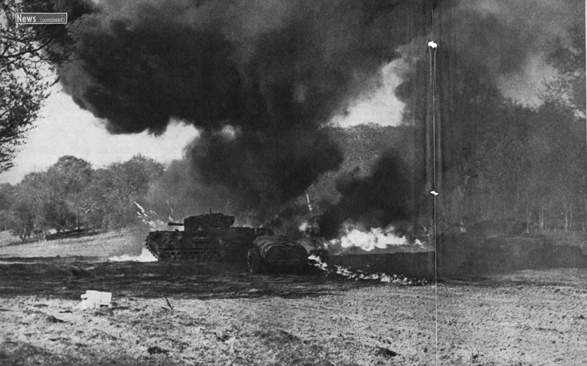
FLAME-THROWING CHURCHILL TANK WHICH HAS BEEN NAMED "CROCODILE" MUST TOW A TRAILER TO PROVIDE FUEL FOR ITS WEAPON. A HIGH-VELOCITY 75 WITH MUZZLE BRAKE HAS REPLACED THE SIX-POUNDER
